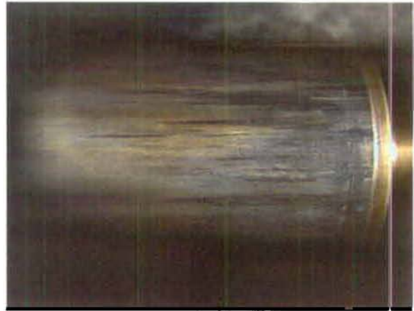
Fig. B: Magnification of scuffing marks (2.6x)
